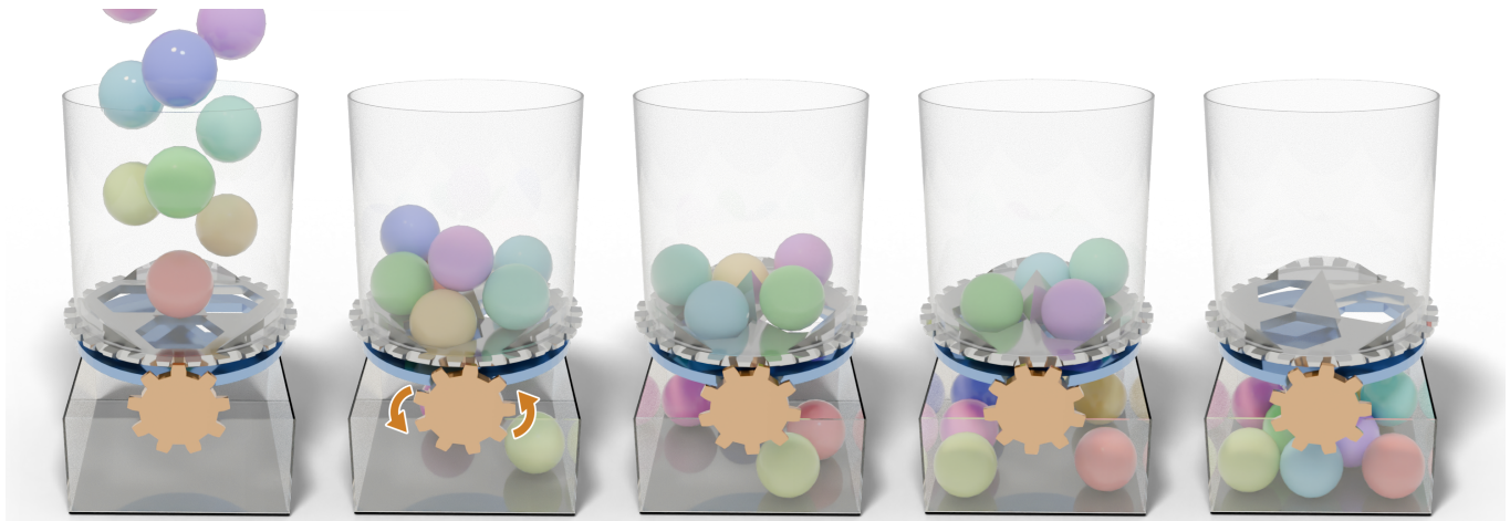
Fig. 1. Gachapon : We simulate the interaction between nine free spheres and a rotating dispenser (silver) driven by a driving gear (orange) using ABD. Throughout the simulation, the non-intersection property is enforced by our proposed CCD algorithm for convex shapes undergoing affine motions. During time steps with peak complexity, our method handles 10 global CCD queries in 16.8 ms, achieving a 12× speed-up than the primitive-based ACCD baseline.
