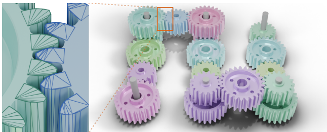
Fig. 10. Gears : A chain of 14 gears driven by the driver gear on the lower-left corner. Each tooth of a gear's collision shape is modeled convex. Our C^5D -Linear method delivers a 14\times speed-up over the ACCD baseline in this scene.
